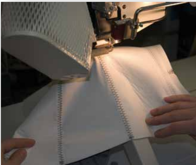
Gore-Tex membrane for waterproof boots is welded. A narrow sealing strip is applied to all seams of the multi-layer lining at around 360 degrees.
